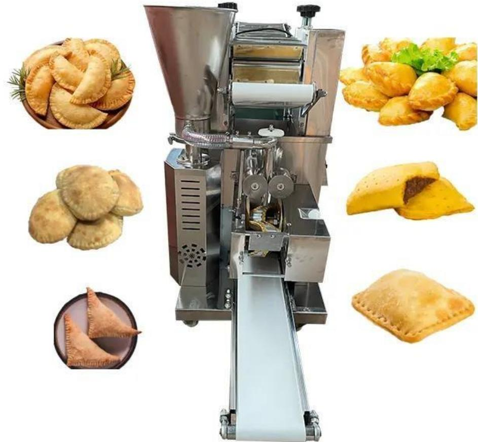
This machine simulates the molding of handmade pastry and, in accordance with the requirements of the pastry process, minimizes friction with the dough to ensure that the empanadas have a smooth and elastic texture.
